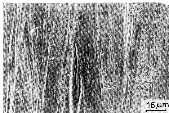
Fig. 3. Microstructure of directionally solidified p -phenylenediamine- m -nitrobenzoic acid eutectic-1 containing 0.82 mole fraction of p -phenylenediamine (X480).
